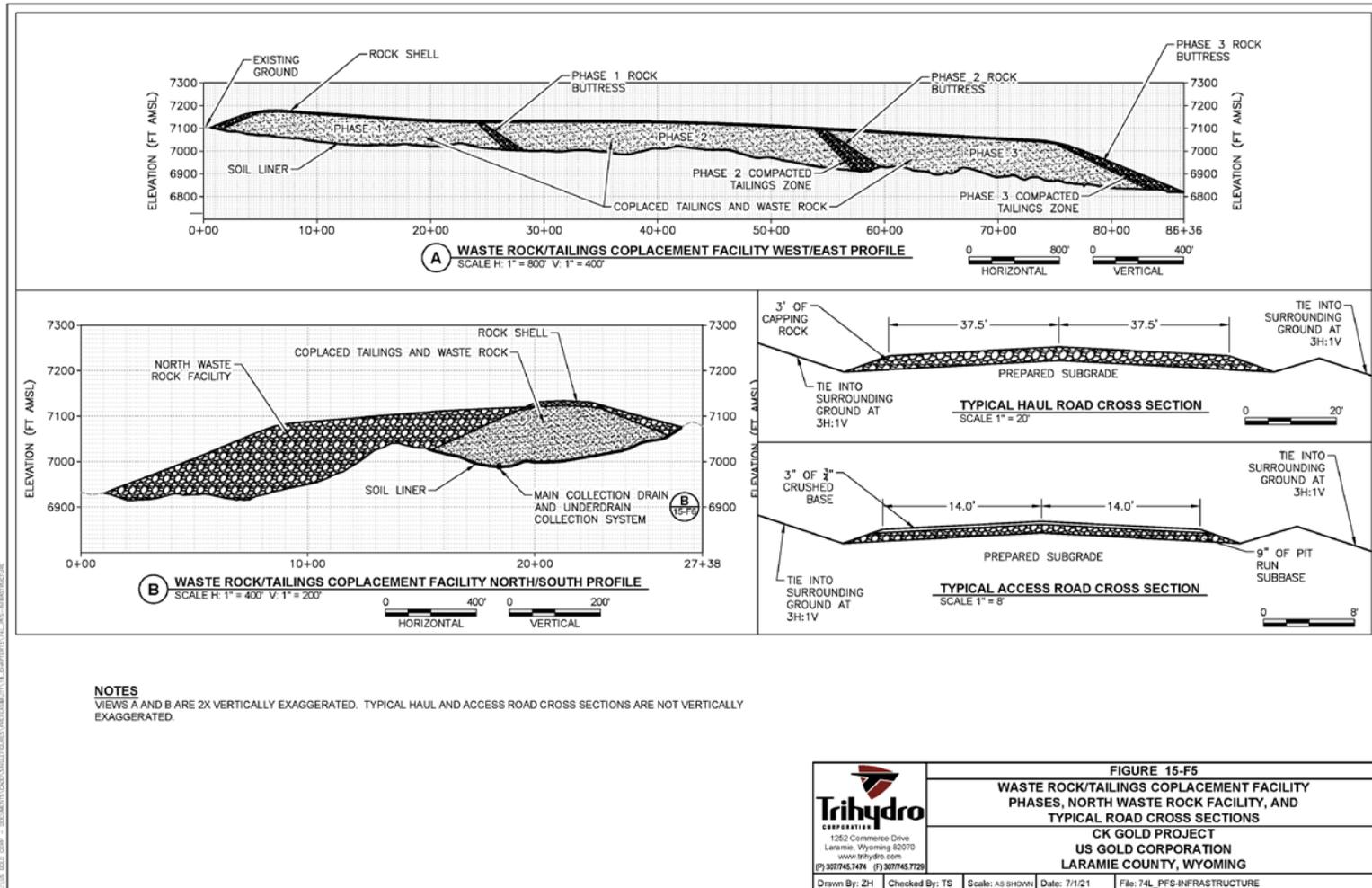
Figure 15-5 Facility Cross Sections
