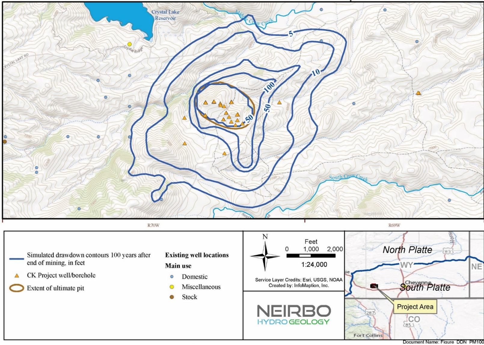
**Figure 13-6 Predicted groundwater drawdown 100 years after mining ends**
