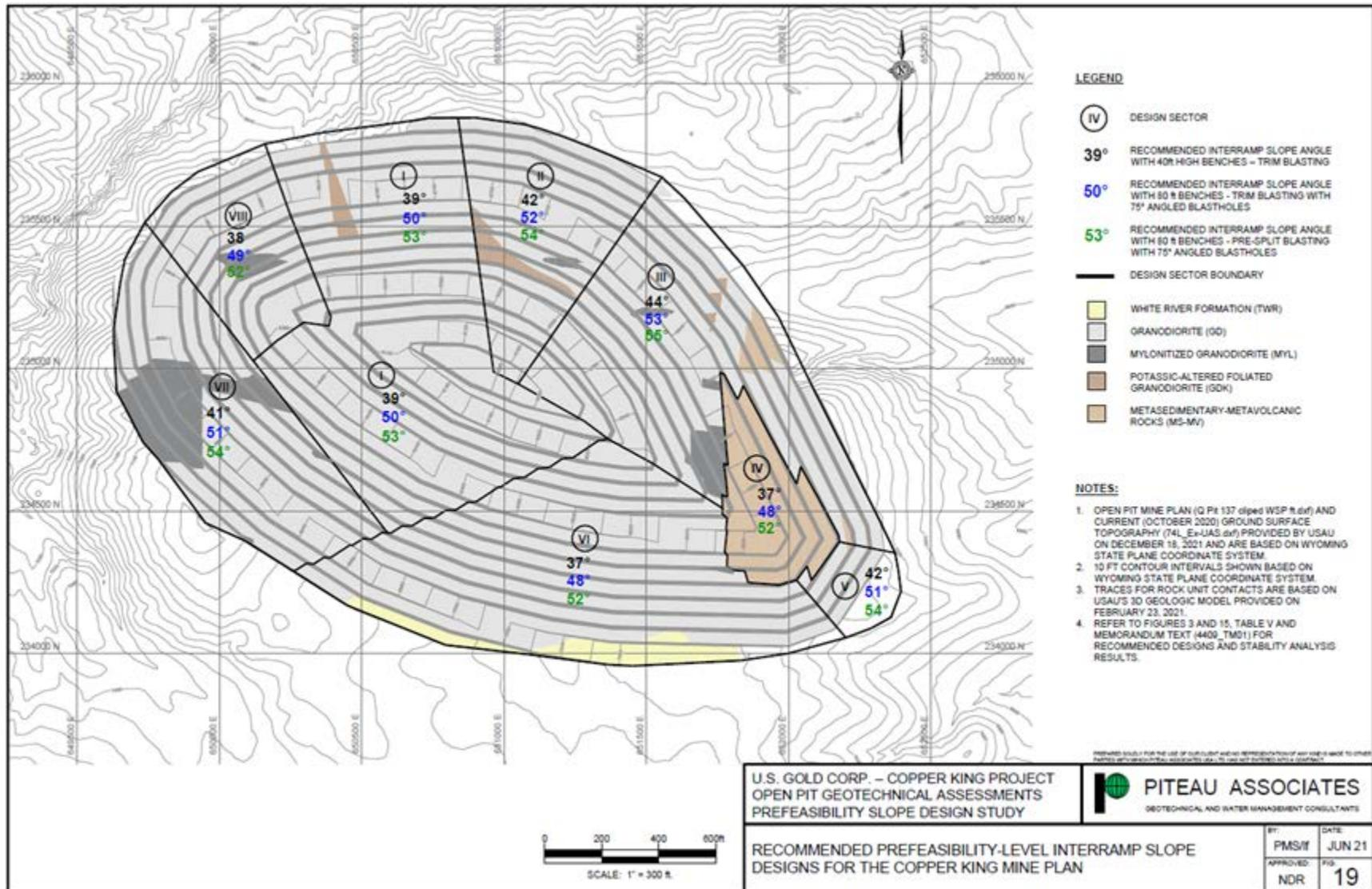
Figure 13-1 Pit Sectors and Recommended Slopes
