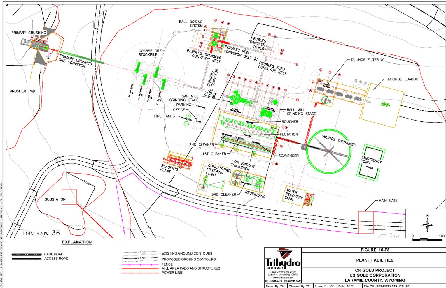
Figure 15-8 Concentrator Plan View
