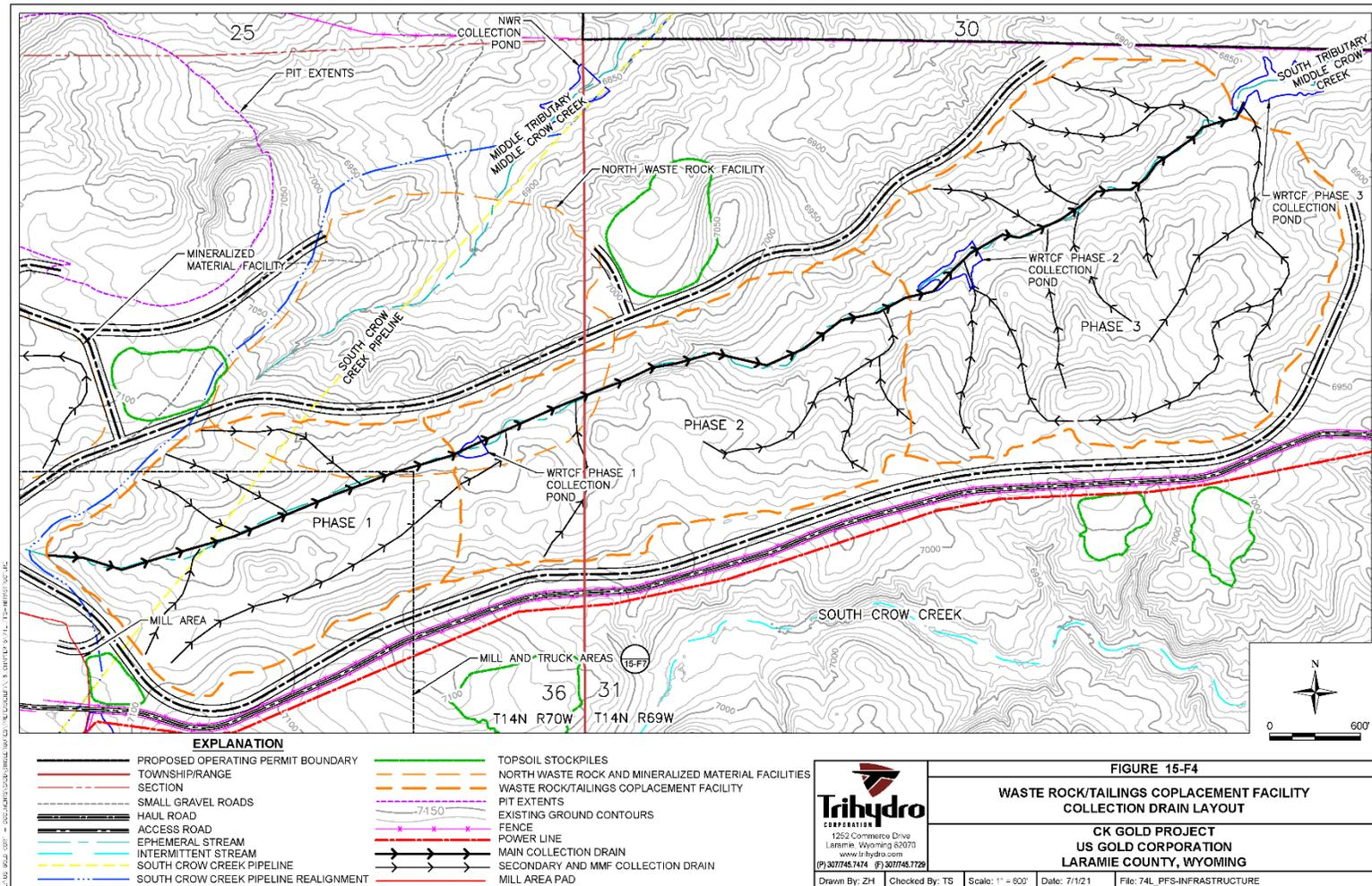
Figure 15-4 WRTCF Collection Drain Layout
