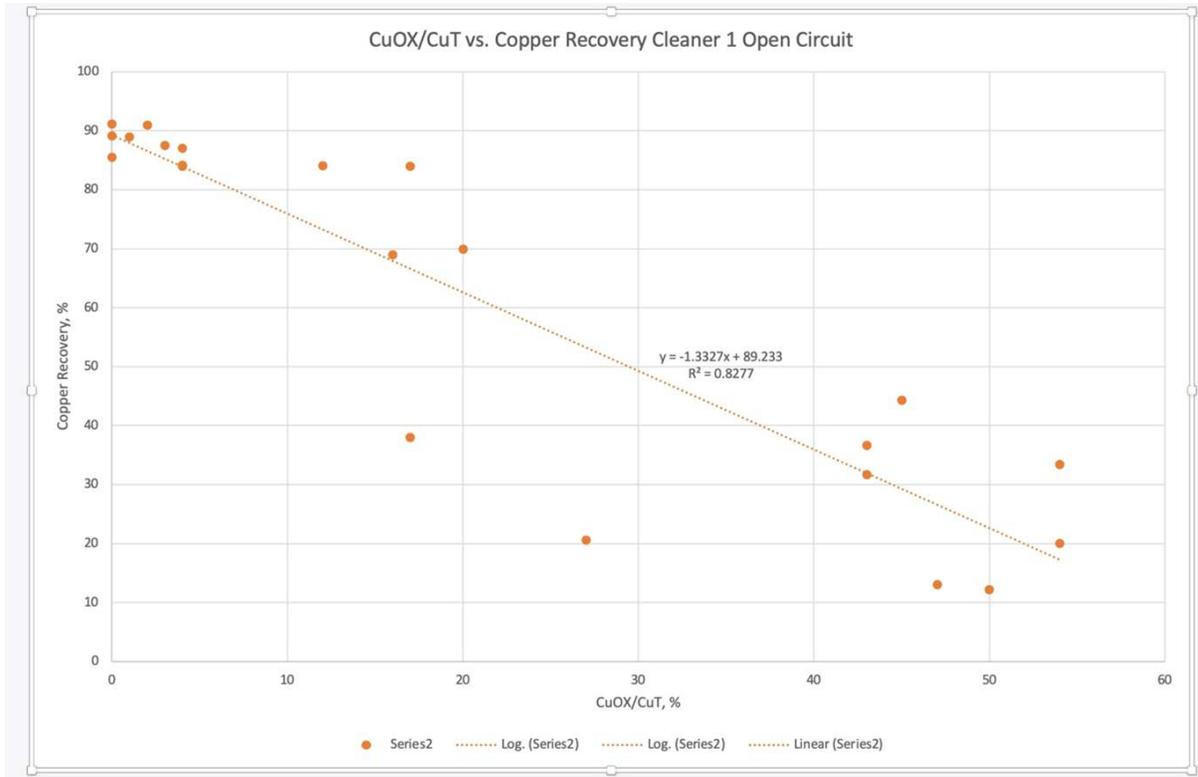
**Figure 10-3 Variability Samples, Copper Recovery v CuOx/CuT**
